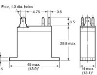
**Mounting Holes** (BOTTOM VIEW) Tolerance: ±0.1 mm
