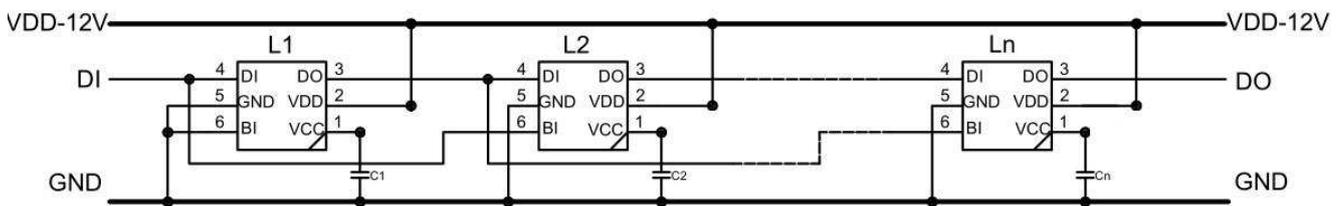
Remarks: C1 is bypass filter capacitor, its value of 100NF.
