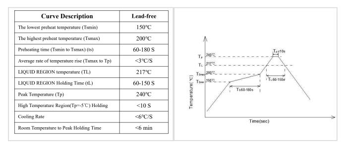
Remarks: 1. These general guidelines may not apply to all PCB designs and reflow soldering configurations.
