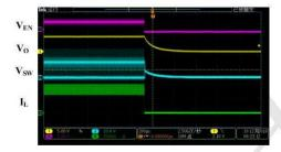
Short Circuit Protection Vin=12V, Vout=5.0V, Lout=800mA - Short
