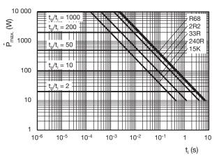
AC10 and AC10-AT Pulse on a regular basis; max. permissible peak pulse power ( $\hat{P}_{max.}$ ) as a function of pulse duration (t<sub>i</sub>)
