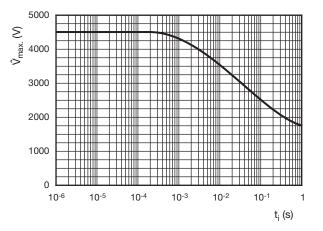
AC10 and AC10-AT Pulse on a regular basis; max. permissible peak pulse voltage (V  $_{max.}$ ) as a function of pulse duration (t<sub>i</sub>)
