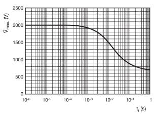
AC05 and AC05-AT Pulse on a regular basis; max. permissible peak pulse voltage (V max.) as a function of pulse duration (t<sub>i</sub>)
