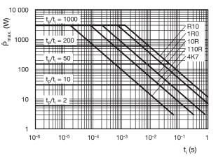
**AC03 and AC03-AT** Pulse on a regular basis; max. permissible peak pulse power ( $\hat{P}_{max.}$ ) as a function of pulse duration (t<sub>i</sub>)
