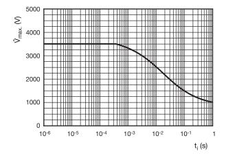
AC07 and AC07-AT Pulse on a regular basis; max. permissible peak pulse voltage (V  $_{max.}$ ) as a function of pulse duration (t<sub>i</sub>)
