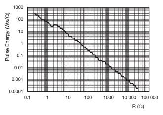
AC10 and AC10-AT Pulse capability; E (Ws) as a function of R ( $\Omega$ )
