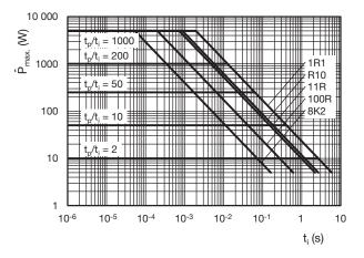
**AC05 and AC05-AT** Pulse on a regular basis; max. permissible peak pulse power ( $\hat{P}_{max.}$ ) as a function of pulse duration (t<sub>i</sub>)
