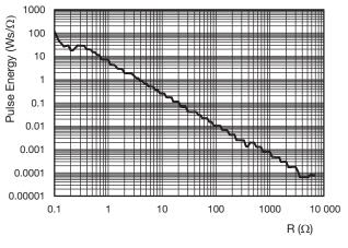
AC03 and AC03-AT Pulse capability; E (Ws) as a function of R ( $\Omega$ )
