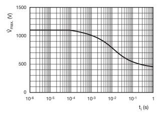
AC01 and AC01-AT Pulse on a regular basis; max. permissible peak pulse voltage ( $\dot{V}_{max.}$ ) as a function of pulse duration ( $t_i$ )
