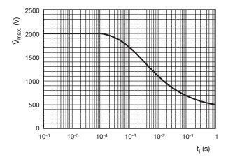
AC04 and AC04-AT Pulse on a regular basis; max. permissible peak pulse voltage (V  $_{max.}$ ) as a function of pulse duration (t<sub>i</sub>)
