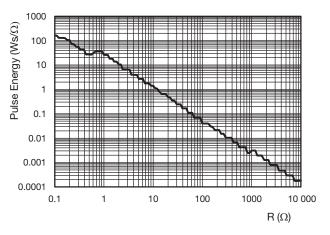
AC05 and AC05-AT Pulse capability; E (Ws) as a function of R ( $\Omega$ )
