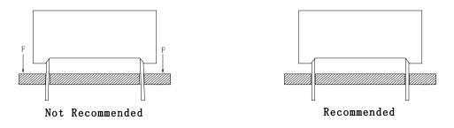
3. The component shall be placed at least 5mm from edge of PCB to avoid damage caused excessive heat during wave soldering.
