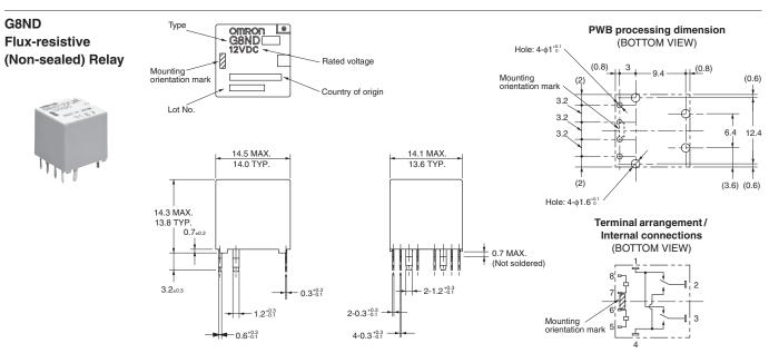
$^{\star}$  Tolerance unless otherwise specified Less than 1 mm:  $\pm 0.1$  mm Less than 1 to 3 mm:  $\pm 0.2$  mm
