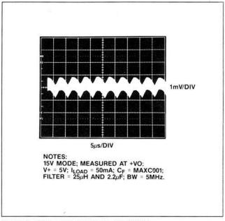
Figure 9. Output Noise Voltage with Pi Filter
