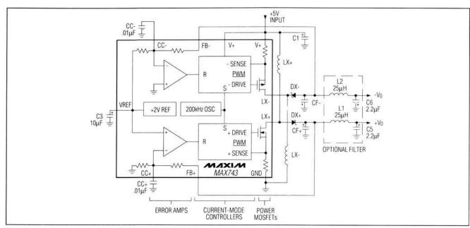
Figure 4. Functional Diagram with Optional Pi Filter
