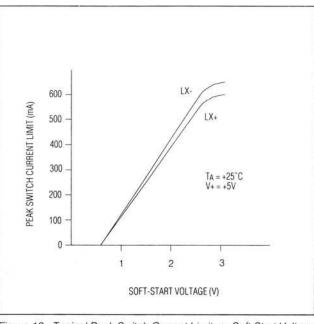
Figure 10. Typical Peak Switch Current Limit vs. Soft-Start Voltage
