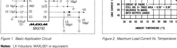
100μF low-ESR equivalent. C1 Bypass Capacitor: MAXC001 or 22µF 16V Tantalum or equivalent.
