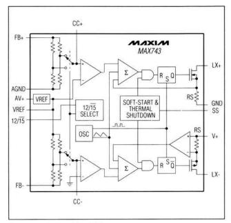
Figure 3. MAX743 Block Diagram
