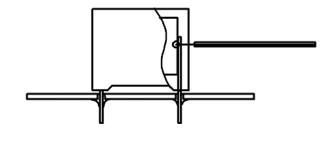
Temperature monitored inside the capacitor.
