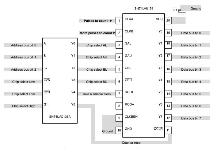
Figure 4. Dual Counter With Address Mapping
