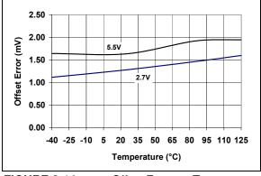
**FIGURE 2-14:** Offset Error vs. Temperature and V<sub>DD</sub>.
