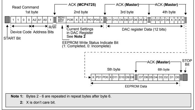
FIGURE 6-3: Read Command and Output Data Format.
