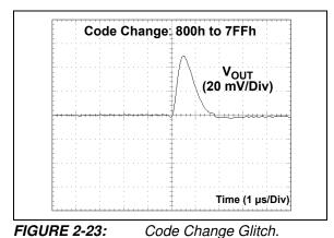
Note: Unless otherwise indicated, T<sub>A</sub> = +25°C, V<sub>DD</sub> = +5.0V, V<sub>SS</sub> = 0V, R<sub>L</sub> = 5 k $\Omega$  to V<sub>SS</sub>, C<sub>L</sub> = 100 pF.
