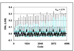
**FIGURE 2-4:** DNL vs. Code and Temperature ( $T_A = -40^{\circ}C$  to  $+125^{\circ}C$ ).
