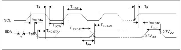
**FIGURE 7-4:**  $l^2C$  Bus Timing Data.
