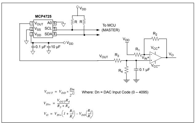
**EXAMPLE 8-3:** Digitally-Controlled Bipolar Voltage Source.
