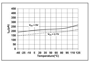
FIGURE 2-11: I<sub>DD</sub> vs. Temperature.
