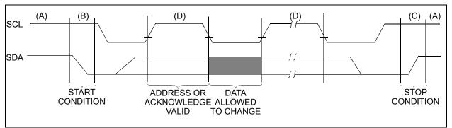
FIGURE 7-3: Data Transfer Sequence On The Serial Bus.
