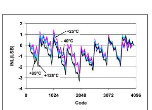
**FIGURE 2-6:** INL vs. Code and Temperature ( $V_{DD} = 5.5V$ ).
