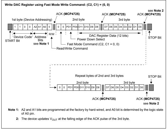
FIGURE 6-1: Fast Mode Write Command.
