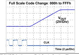
FIGURE 2-19: Full Scale Settling Time.
