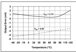
**FIGURE 2-10:** Output Error vs. Temperature (Code = 4000d).
