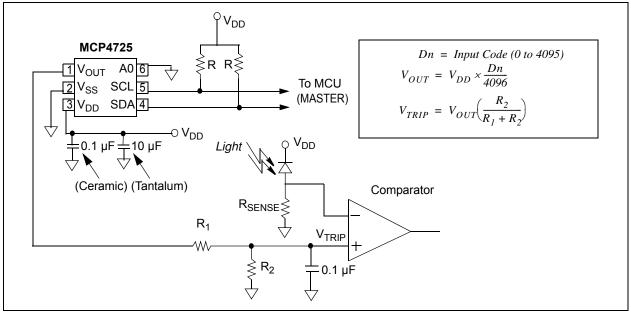
**EXAMPLE 8-1:** Set Point Or Threshold Calibration.
