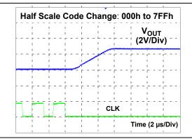
FIGURE 2-21: Half Scale Settling Time.
