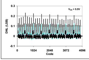
**FIGURE 2-2:** DNL vs. Code and Temperature ( $T_A = -40^{\circ}C$  to  $+125^{\circ}C$ ).
