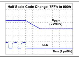
FIGURE 2-22: Half Scale Settling Time.
