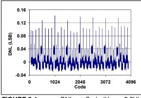
FIGURE 2-1: DNL vs. Code ( $V_{DD} = 5.5V$ ).
