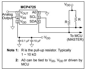
**FIGURE 8-1:**  $l^2C$  Bus Interface Connection with A0 pin tied to  $V_{SS}$ .
