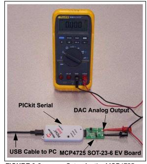
**FIGURE 9-2:** Setup for the MCP4725 SOT-23-6 Evaluation Board with PICkit<sup>™</sup> Serial Analyzer.
