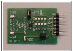
FIGURE 9-1: MCP4725 SOT-23-6 Evaluation Board.
