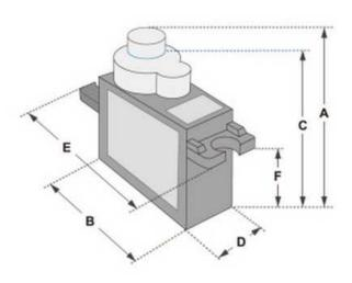
Position "0" (1.5 ms pulse) is middle, "90" (~2ms pulse) is middle, is all the way to the right, "-90" (~1ms pulse) is all the way to the left.
