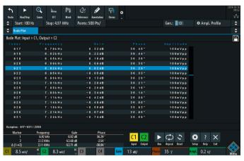
A table of measurement results provides detailed information about each measurement point, consisting of frequency, gain and phase shift
