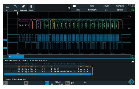
Decoded hexadecimal I<sup>2</sup>C message shown in honeycomb format and in table
