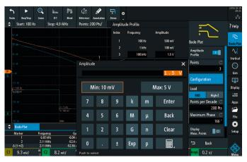
The amplitude output level of the generator signal can be varied during the measurement to suppress the noise behavior of the DUT
