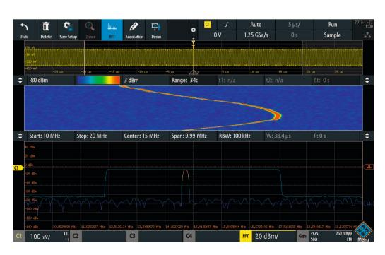
Test signal from three different perspectives: time domain (top), spectrogram (center) and frequency domain (bottom)
