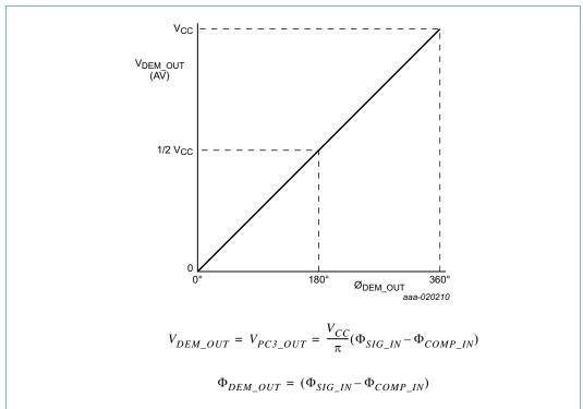
Fig 10. Phase comparator 3; average output voltage as a function of input phase difference
