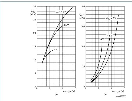
To obtain optimum temperature stability, C1 must be as small as possible but larger than 100 pF. (a) R1 = 3 k $\Omega$ ; C1 = 40 pF (b) R1 = 3 k $\Omega$ ; C1 = 100 nF
