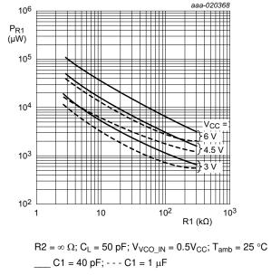
Fig 24. Power dissipation as a function of R1
