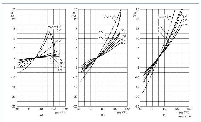
To obtain optimum temperature stability, C1 must be as small as possible but larger than 100 pF.
