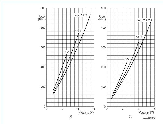
To obtain optimum temperature stability, C1 must be as small as possible but larger than 100 pF. (a) R1 = 300 k $\Omega$ ; C1 = 40 pF (b) R1 = 300 k $\Omega$ ; C1 = 100 nF
