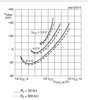
Fig 15. Offset voltage at demodulator output as a function of VCO\_IN and R<sub>s</sub>
