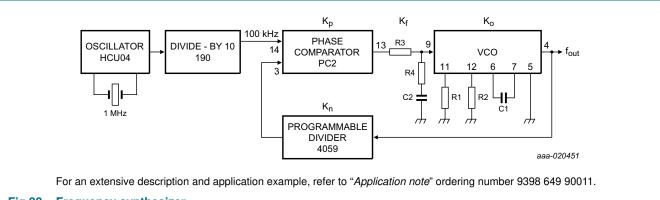
Fig 33. Frequency synthesizer
