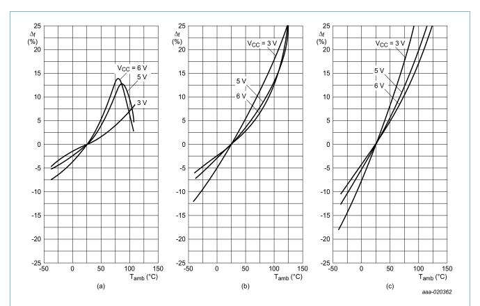
To obtain optimum temperature stability, C1 must be as small as possible but larger than 100 pF.
