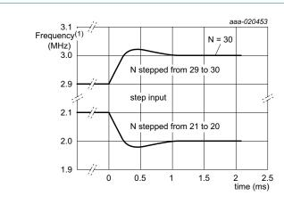
The output frequency is proportional to the VCO control voltage. As a result, the PLL frequency response can be observed with an oscilloscope by monitoring pin VCO\_IN of the VCO. The average frequency response, as calculated by the Laplace method, is found experimentally by smoothing this voltage at pin VCO\_IN using a simple RC filter. The filter has a long time constant when compared with the phase detector sampling rate but short when compared with the PLL response time.
