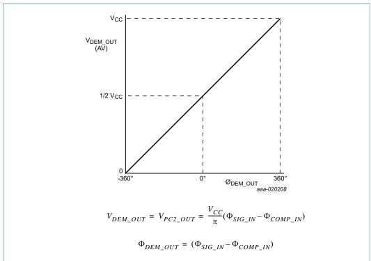
Fig 8. Phase comparator 2; average output voltage as a function of input phase difference
