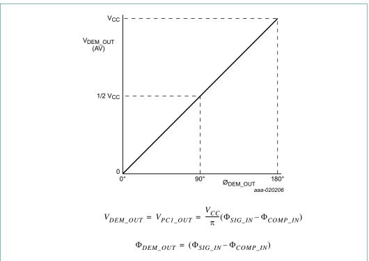
Fig 6. Phase comparator 1; average output voltage as a function of input phase difference
