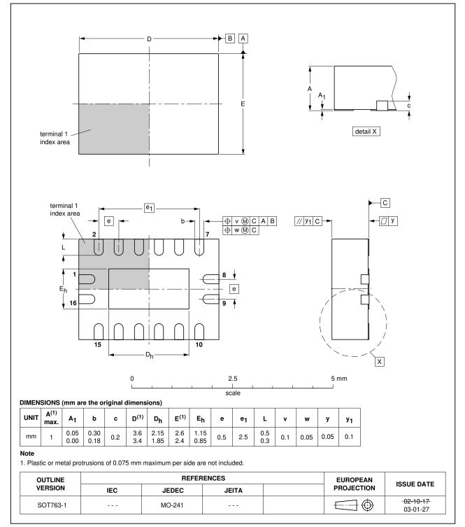
DHVQFN16: plastic dual in-line compatible thermal enhanced very thin quad flat package; no leads; 16 terminals; body 2.5 x 3.5 x 0.85 mm SOT763-1
