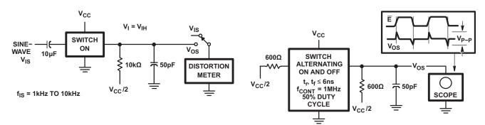
Figure 12. ¼Sine-Wave Distortion Test Circuit
