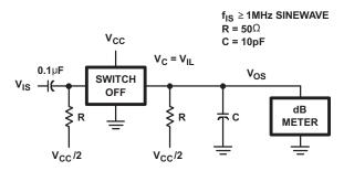
Figure 14. Switch OFF Signal Feedthrough
