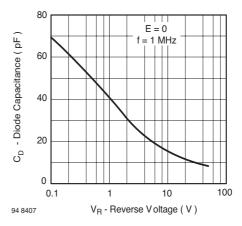
Figure 6. Diode Capacitance vs. Reverse Voltage
