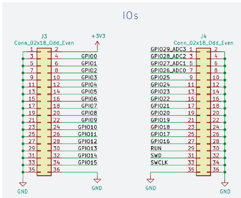
Figure 10. Schematic section showing the 2.54mm IO headers
