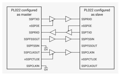
Figure 100 shows how an PrimeCell SSP (PL022), configured as master, interfaces to a Motorola SPI slave. The SPI Slave Select (SS) signal is permanently tied LOW and configures it as a slave. Similar to the above operation, the master can broadcast to the slave through the master PrimeCell SSP SSPTXD line. In response, the slave drives its SPI MISO port onto the SSPRXD line of the master.
