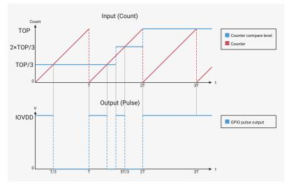
The behaviour becomes even more perplexing if the TOP register is also modified. It would be difficult for software to write to CC or TOP with the correct timing. To solve this, each slice has two copies of the CC and TOP registers: one copy which software can modify, and another, internal copy which is updated from the first register at the instant the counter wraps. Software can modify its copy of the register at will, but the changes are not captured by the PWM output until the next wrap.
