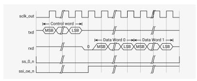
Figure 137. FIFO Status for Sequential Microwire Transfer (receiving data frame)
