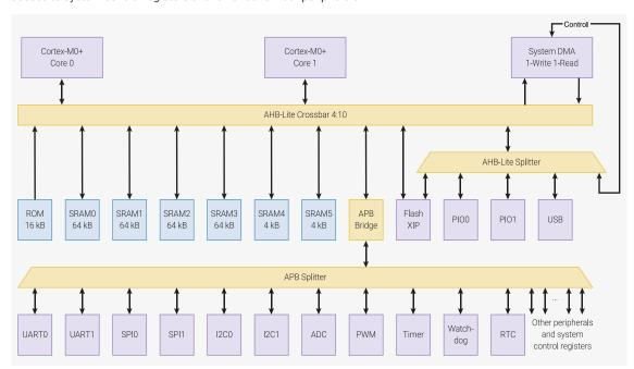
The bus fabric connects 4 AHB-Lite masters, i.e. devices which generate addresses:
