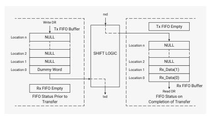
For eeprom\_read transfers (transfer mode field [9:8] of the Control Register 0 = 11b), opcode and/or EEPROM address are written into the transmit FIFO. During transmission of these control frames, received data is not captured by the DW\_apb\_ssi master. After the control frames have been transmitted, receive data from the EEPROM is stored in the receive FIFO.
