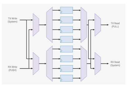
Another example is a UART: because the TX/CTS and RX/RTS parts a of a UART are asynchronous, they are implemented on two separate state machines. It would be wasteful to leave half of each state machine's FIFO resources idle. The ability to join the two halves into just a TX FIFO for the TX/CTS state machine, or just an RX FIFO in the case of the RX/RTS state machine, allows full utilisation. A UART equipped with an 8-deep FIFO can be left alone for
