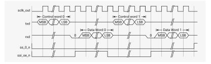
The only modification needed to perform a continuous nonsequential transfer is to write more control words into the transmit FIFO buffer; this is illustrated in Figure 135. In this example, two data words are read from the external serial-slave device.
