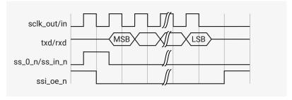
Continuous data frames are transferred in the same way as single data frames. The frame indicator is asserted for one clock period during the same cycle as the LSB from the current transfer, indicating that another data frame follows.
