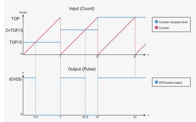
In Figure 108, the input value only changes at the instant where the counter wraps through 0. Figure 109 shows what happens if the input value is allowed to change at any other time: an unwanted glitch is produced at the output.
