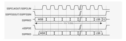
Figure 91 shows a continuous transmission signal sequence for Motorola SPI frame format with SPO=0, SPH=0.
