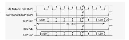
Figure 94 shows a continuous transmission signal sequence for Motorola SPI format with SPO=1, SPH=0.
