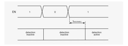
Detection is re-enabled if the BOD register is reset, as this sets the register's EN field to one. Again, detection will become active after a delay equal to the brown-out detection enable delay (t<sub>BOD.ENABLE</sub>).
