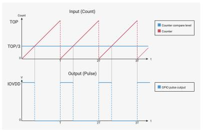
This example shows the counting period and the A and B counter compare levels being configured on one of RP2040's PWM slices.
