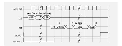
Figure 133 shows how the data and control frames are structured in the transmit FIFO prior to the transfer; the value programmed into the MWCR register is also shown.
