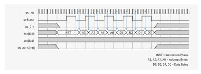
Figure 160. Transmit Data With DDR\_DRIVE\_EDGE = 2
