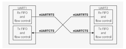
When the RTS flow control is enabled, nUARTRTS is asserted until the receive FIFO is filled up to the programmed watermark level. When the CTS flow control is enabled, the transmitter can only transmit data when nUARTCTS is asserted.
