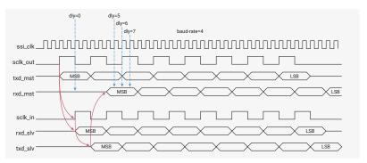
The Slave uses the sclk\_out signal from the master as a strobe in order to drive rxd signal data onto the serial bus. Routing and sampling delays on the sclk\_out signal by the slave device can mean that the rxd bit has not stabilized to the correct value before the master samples the rxd signal. Figure 119 shows an example of how a routing delay on the rxd signal can result in an incorrect rxd value at the default time when the master samples the port.
