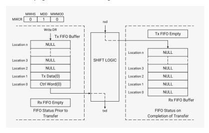
Continuous transfers occur as shown in Figure 140, with the control word for the next transfer following immediately after the LSB of the current data word.
