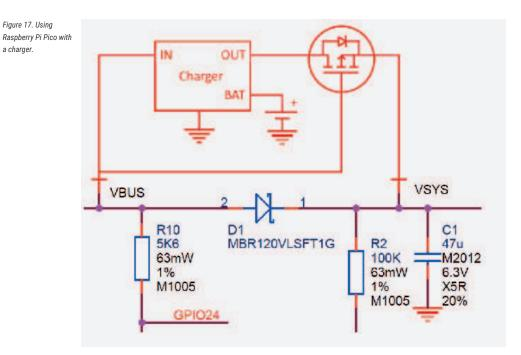
In the example we feed VBUS to the input of the charger, and we feed VSYS with the output via the previously mentioned P-FET arrangement. Depending on your use case you may also want to add a schottky diode across the P-FET as described in the previous section.
