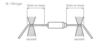
The tensile strength applied to the lead wire should be 49N or less for SF-type and 9.8N or less for SM-types. The strength applied to the body of the thermal link should be 98N or less for SF-type, 49N or less for SM-type.
