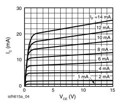
Fig. 3 - Switching Operation (with saturation)
