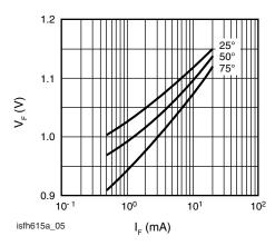
Fig. 6 - Diode Forward Voltage (typ.) vs. Forward Current
