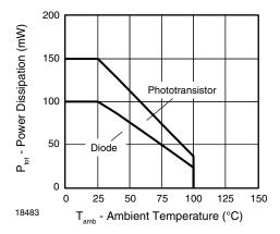
Fig. 1 - Permissible Power Dissipation vs. Ambient Temperature
