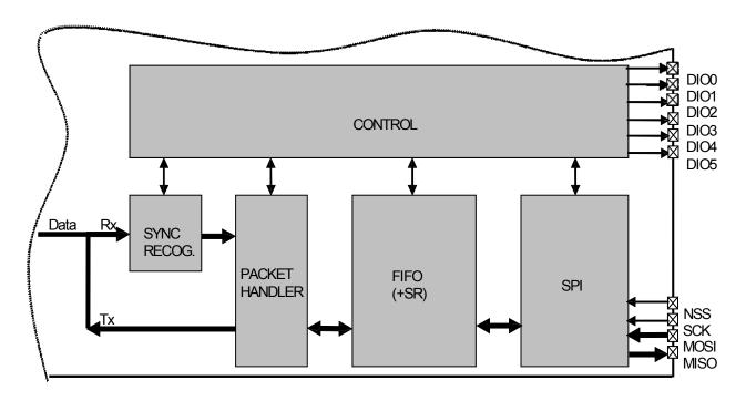
Figure 32. Packet Mode Conceptual View
