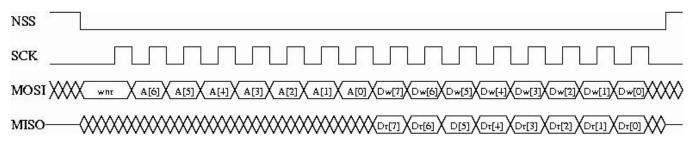
Figure 25. SPI Timing Diagram (single access)
