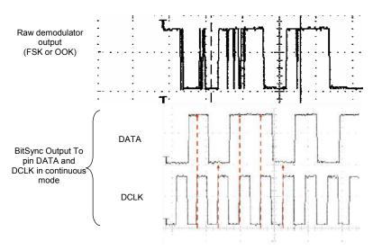
Figure 13. Bit Synchronizer Description
