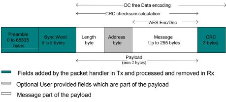
Figure 34. Variable Length Packet Format
