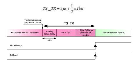
Figure 17. Tx Startup, FSK and OOK
