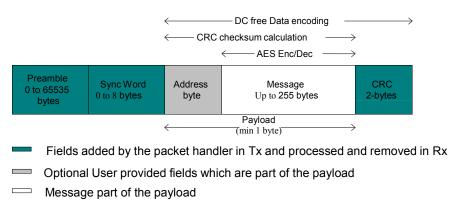
Figure 33. Fixed Length Packet Format
