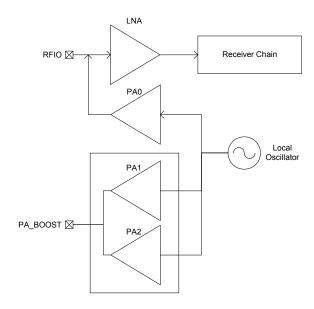
Figure 5. Transmitter Block Diagram
