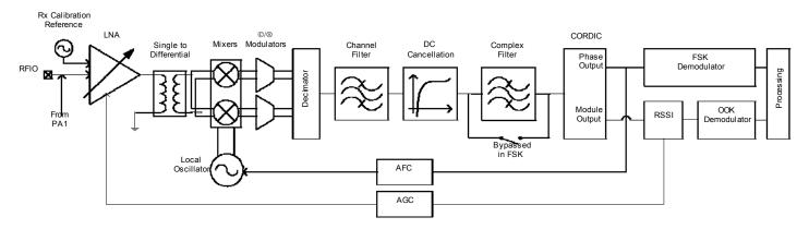
Figure 7. Receiver Block Diagram
