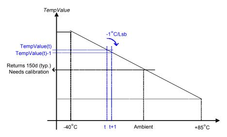
Figure 16. Temperature Sensor Response
