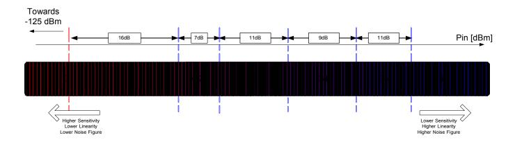
Figure 8. AGC Thresholds Settings
