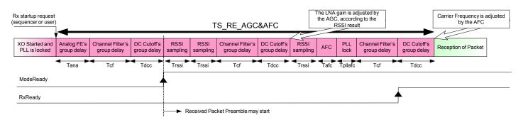
Figure 20. Rx Startup - AGC and AFC
