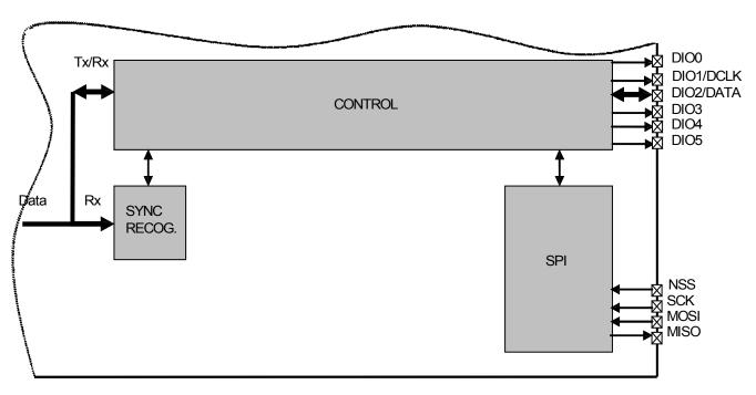
Figure 29. Continuous Mode Conceptual View
