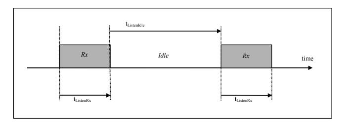
Figure 21. Listen Mode Sequence (no wanted signal is received)
