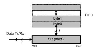
Figure 26. FIFO and Shift Register (SR)
