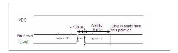
Figure 40. Manual Reset Timing Diagram
