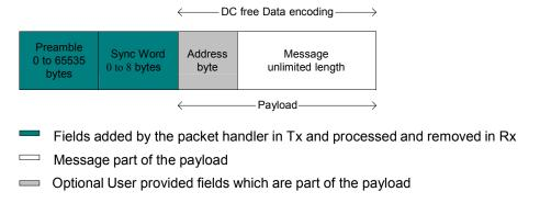
Figure 35. Unlimited Length Packet Format
