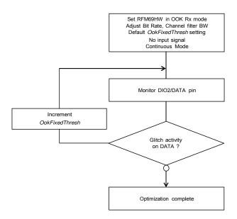
Figure 12. Floor Threshold Optimization
