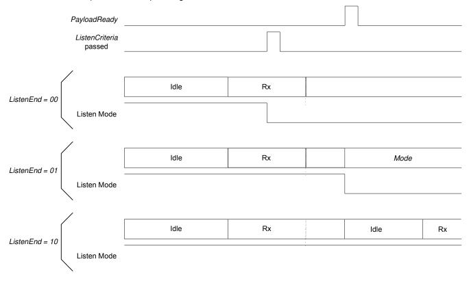
Figure 22. Listen Mode Sequence (wanted signal is received)
