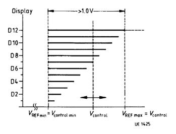
If a quartet does not need the full number of display diodes and if the first connected diodes shall be left luminous at full driving, bridges have to be inserted replacing the missing LEDs. Otherwise the first diodes of the quartet switch off when their display range is exceeded.
