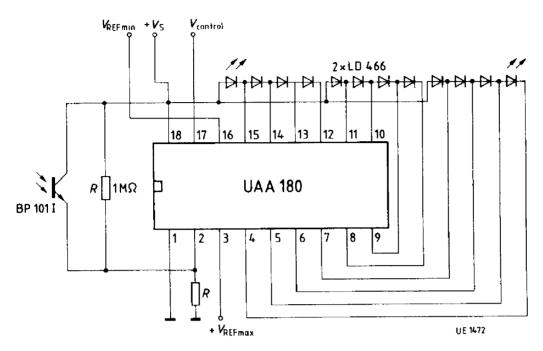
$R = 2.2 \text{ k}\Omega...100 \text{ k}\Omega$
