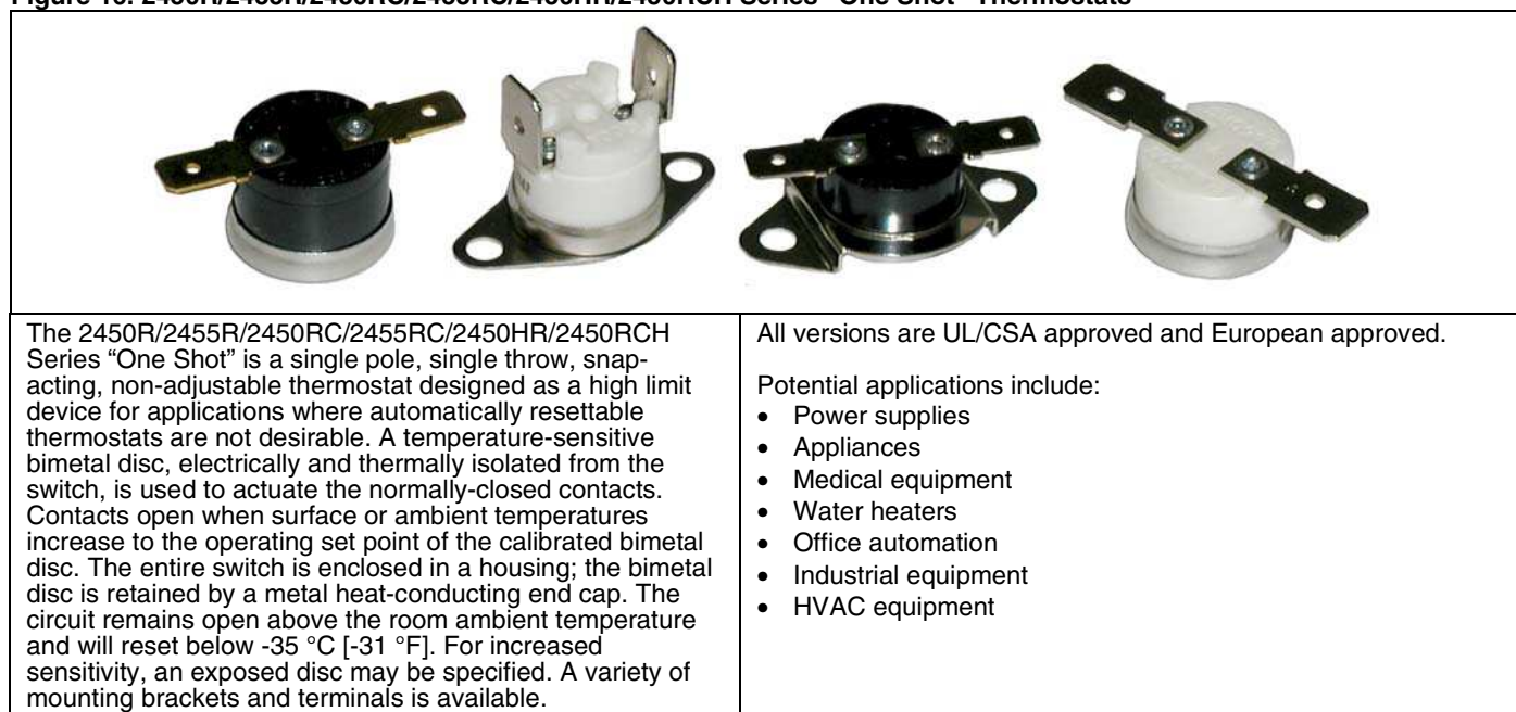
Figure 16. 2450R/2455R/2450RC/2455RC/2450HR/2450RCH Series “One Shot” Thermostats
