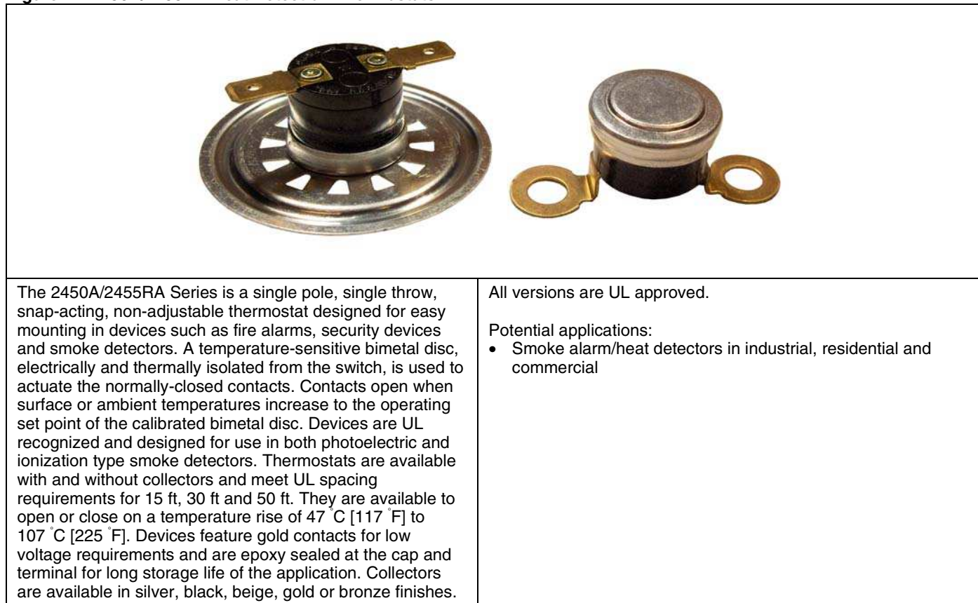
Figure 12. 2450A/2455RA Heat Detection Thermostats
