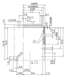
Q indicates the center line of the microSD card slot. 2
