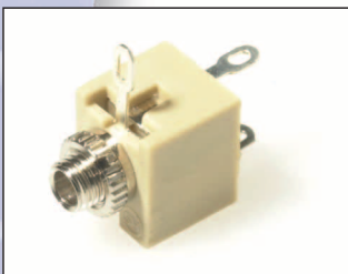
JYO-35 mono switched 3.5mm Jack Socket. Panel mounting with solder tags. Supplied with ring nut.
