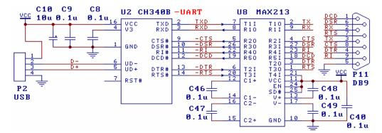
The image above use CH340T/CH340B (or CH340C) to realize USB to RS232 converter. CH340 provides common UART and MODEM signal, converts TTL to RS232 through level conversion chip U8. Port P11 is DB9 connector, the pin and its function are the same as common PC DB9 connector, the chips similar with U8 have MAX213/ADM213/SP213/MAX211 etc.
