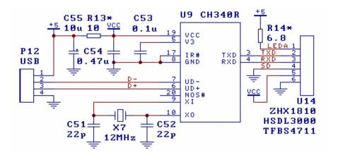
The image above is USB to infrared adapter design is composed with USB convert IrDA infrared chip CH340R and infrared transceiver U14 (ZHX1810/HSDL3000 etc). The resistor R13 is used to weaken influence of large current in infrared transmitting. The current limiting resistor R14 should be adjusted according to the manufacturer's recommended value of the infrared transceiver U14.
