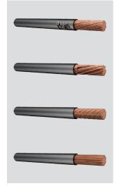
The conductor insulation has been damaged by the stripping tool
