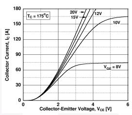
**Figure 4. Transfer Characteristics**
