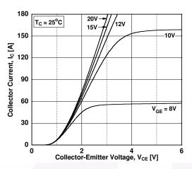
Figure 3. Typical Saturation Voltage Characteristics
