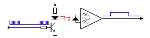
Infrared emitting diode launch out the modulation signal and infrared receiver head will receive, decode, filter and so on to regain the signal.
