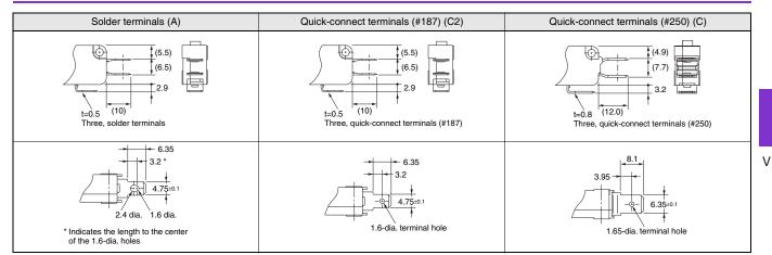
Note. The above is for the SPDT contact specifications. Two terminals will be available for SPST-NO or SPST-NC contact specifications. For terminal positions, refer to Contact form on page 9.
