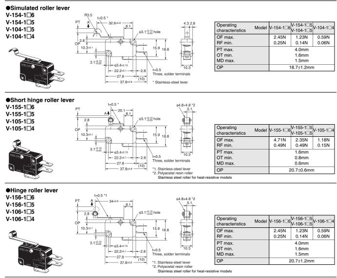
Note 1. Unless otherwise specified, a tolerance of  $\pm 0.4$  mm applies to all dimensions. Note 2. The operating characteristics are for operation in the A direction ( $\clubsuit$ ).
