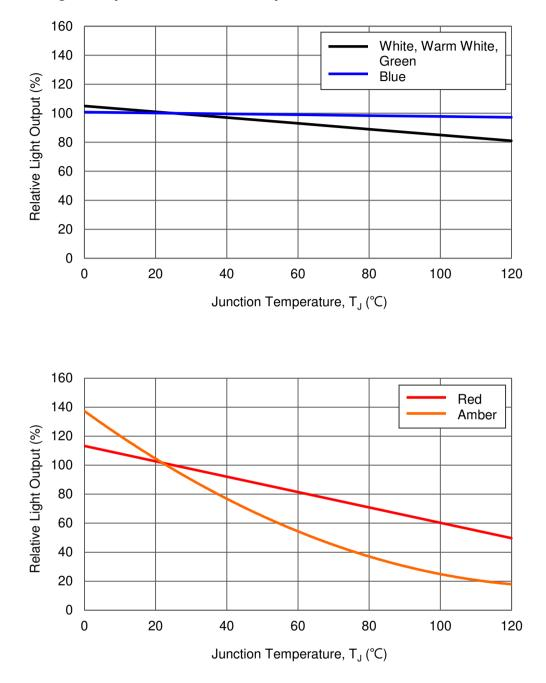
Relative Light Output vs. Junction Temperature at 350mA
