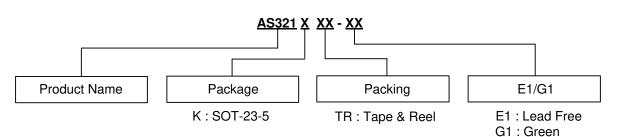
Diodes IC's Pb-free products, as designated with "E1" suffix in the part number, are RoHS compliant. Products with "G1" suffix are available in green packages.
