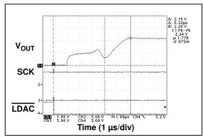
**FIGURE 2-32:** V<sub>OUT</sub> Rise Time Exit Shutdown.
