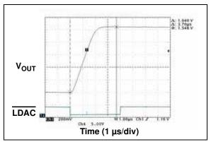
FIGURE 2-31:  $V_{OUT}$  Rise Time.
