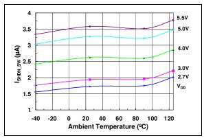
**FIGURE 2-18:** Software Shutdown Current vs. Temperature and  $V_{DD}$ .
