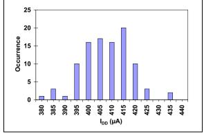
**FIGURE 2-16:**  $I_{DD}$  Histogram ( $V_{DD} = 2.7V$ ).
