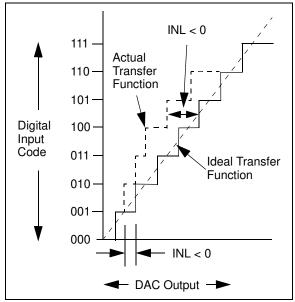
FIGURE 4-1: Example for INL Error.
