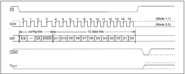
FIGURE 5-1: Write Command for MCP4822 (12-bit DAC).
