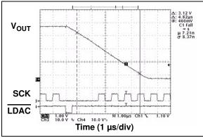
FIGURE 2-29: V<sub>OUT</sub> Fall Time.
