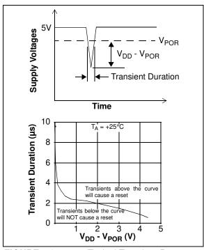
FIGURE 4-3: Typical Transient Response.
