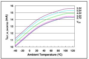
**FIGURE 2-26:**  $I_{OUT}$  High Short vs. Temperature and  $V_{DD}$ .
