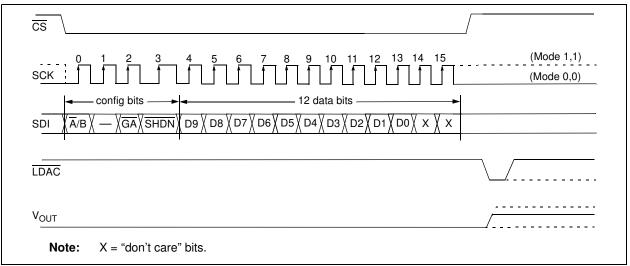
FIGURE 5-2: Write Command for MCP4812 (10-bit DAC).
