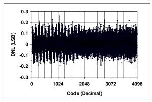
FIGURE 2-1: DNL vs. Code (MCP4822).
