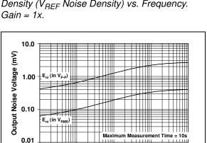
**FIGURE 2-14:** Output Noise Voltage  $(V_{REF} Noise Voltage) vs. Bandwidth. Gain = 1x.$
