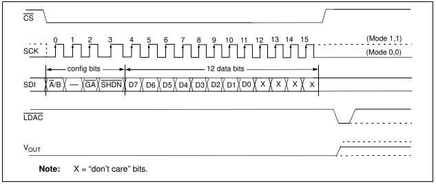
FIGURE 5-3: Write Command for MCP4802 (8-bit DAC).
