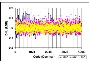
FIGURE 2-2: DNL vs. Code and Temperature (MCP4822).
