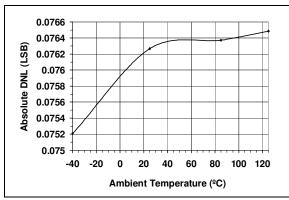
**FIGURE 2-3:** Absolute DNL vs. Temperature (MCP4822).
