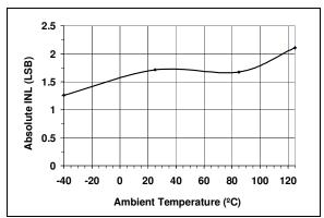
FIGURE 2-5: Absolute INL vs. Temperature (MCP4822).
