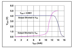
**FIGURE 2-27:**  $I_{OUT}$  vs.  $V_{OUT}$ . Gain = 2x.
