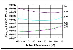
**FIGURE 2-25:**  $V_{OUT}$  Low Limit vs. Temperature and  $V_{DD}$ .
