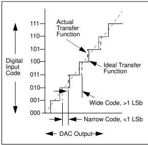
FIGURE 4-2: Example for DNL Error.
