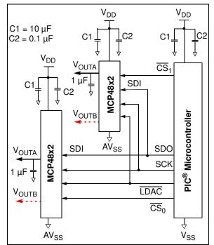
**FIGURE 6-1:** Typical Connection Diagram.
