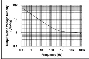
**FIGURE 2-13:** Output Noise Voltage Density (V<sub>REF</sub> Noise Density) vs. Frequency.
