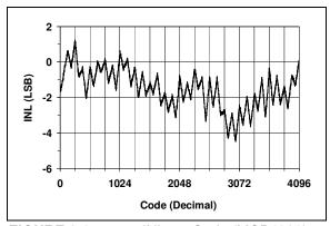
FIGURE 2-6: INL vs. Code (MCP4822).
