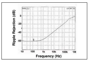
FIGURE 2-33: PSRR vs. Frequency.
