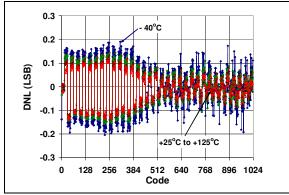
FIGURE 2-7: DNL vs. Code and Temperature (MCP4812).
