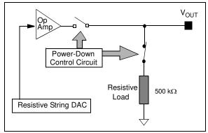
FIGURE 4-4: Output Stage for Shutdown Mode.
