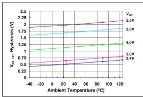
**FIGURE 2-23:** Input Hysteresis vs. Temperature and  $V_{DD}$ .
