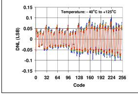
FIGURE 2-9: DNL vs. Code and Temperature (MCP4802).
