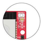
**STATUS** LED turns on when the firmware is running
