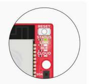
LINK LED remains turned on when your FLUO WI-FI is connected to your wireless network
