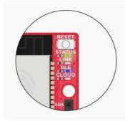
**BLE** LED blinks when the Bluetooth connection on your FLUO WI-FI is in discoverable mode
