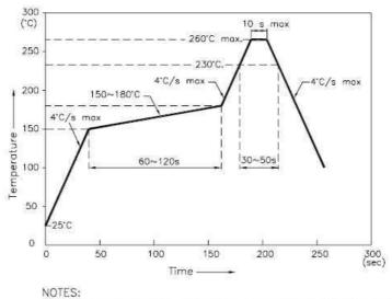
Reflow Soldering Profile For Lead-free SMT Process.
