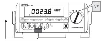
Figure 3-15. Temperature Measurement
