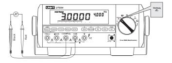
Figure 3-14. Frequency / Duty Cycle Measurement
