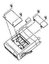
Figure 6-2. Battery Replacement
