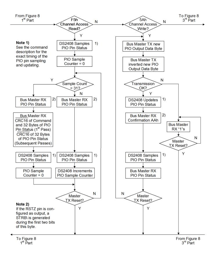
Figure 8-3. CONTROL FUNCTIONS FLOW CHART
