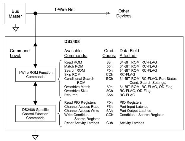
Figure 2. HIERARCHICAL STRUCTURE FOR 1-Wire PROTOCOL
