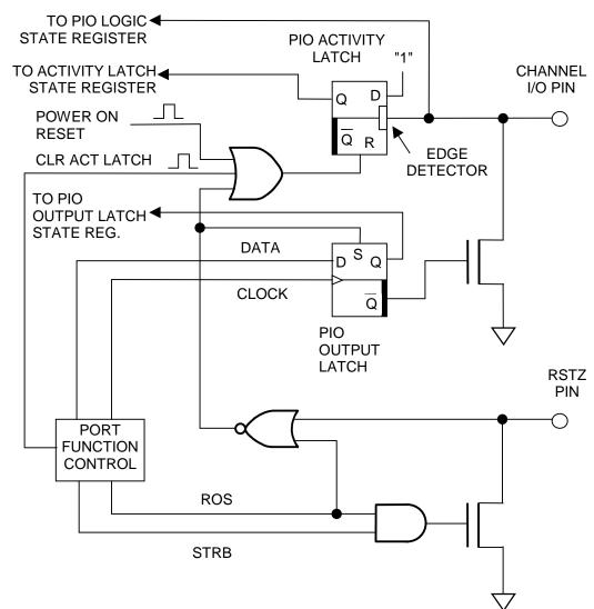
Figure 6. CHANNEL I/O AND RSTZ SIMPLIFIED LOGIC DIAGRAM
