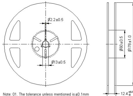
Note: 01. The tolerance unless mentioned is ±0.1mm 02. The measured unit is "mm"
