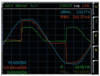
Waveform function: load with phase-angle control.
