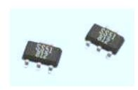
SS5 Series Hall effect position sensors are operated by the magnetic field from a permanent magnet or electromagnet. The small SOT89 style package surface mounts on PC boards and flexible circuits. The SS5 uses a industry standard "gull-wing" design which makes it less susceptible to "solder bridging" and allows increased circuit board density. The SS5 series package can accommodate larger IC's than SS1 and allows for four-pin designs
