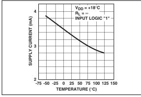
*FIGURE 2-9:* Supply Current vs. Temperature.
