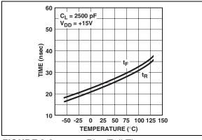
FIGURE 2-2: Rise/Fall Times vs. Temperature.
