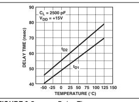
FIGURE 2-5: Delay Times vs. Temperature.
