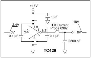
FIGURE 4-4: Peak Output Current Test Circuit.
