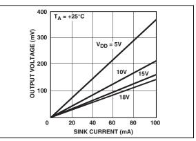
**FIGURE 2-12:** Low Output Voltage vs. Output Sink Current.
