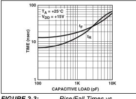
FIGURE 2-3: Rise/Fall Times vs. Capacitive Load.
