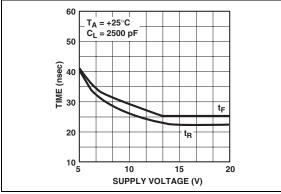
FIGURE 2-1: Rise/Fall Times vs. Supply Voltage.
