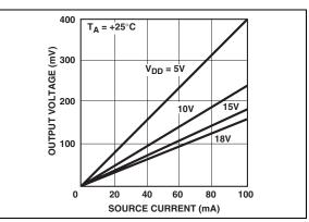
**FIGURE 2-11:** High Output Voltage (V<sub>DD</sub>-V<sub>OH</sub>) vs. Output Source Current.
