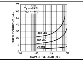
*FIGURE 2-4:* Supply Current vs. Capacitive Load.
