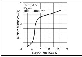
FIGURE 2-8:Supply Current vs. SupplyVoltage.
