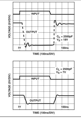
FIGURE 4-2: Switching Speed.
