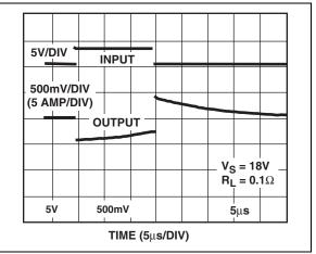
FIGURE 4-5: Peak Output Current Capability.
