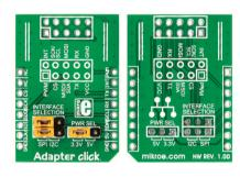
Adapter Click™ is an accessory board in **mikroBUS™** form factor. It's a compact and easy solution for adding mikroBUS™ to IDC10 adapter to your design. It features 2x5 connection pads and two jumpers for SPI/I²C selection. Adapter Click™ communicates with the target board microcontroller via **mikroBUS™** I²C (SDA, SCL), SPI (MISO, MOSI, SCK, CS), UART (RX, TX), INT and PWM lines. The board is designed to use 3.3V and 5V power supply.
