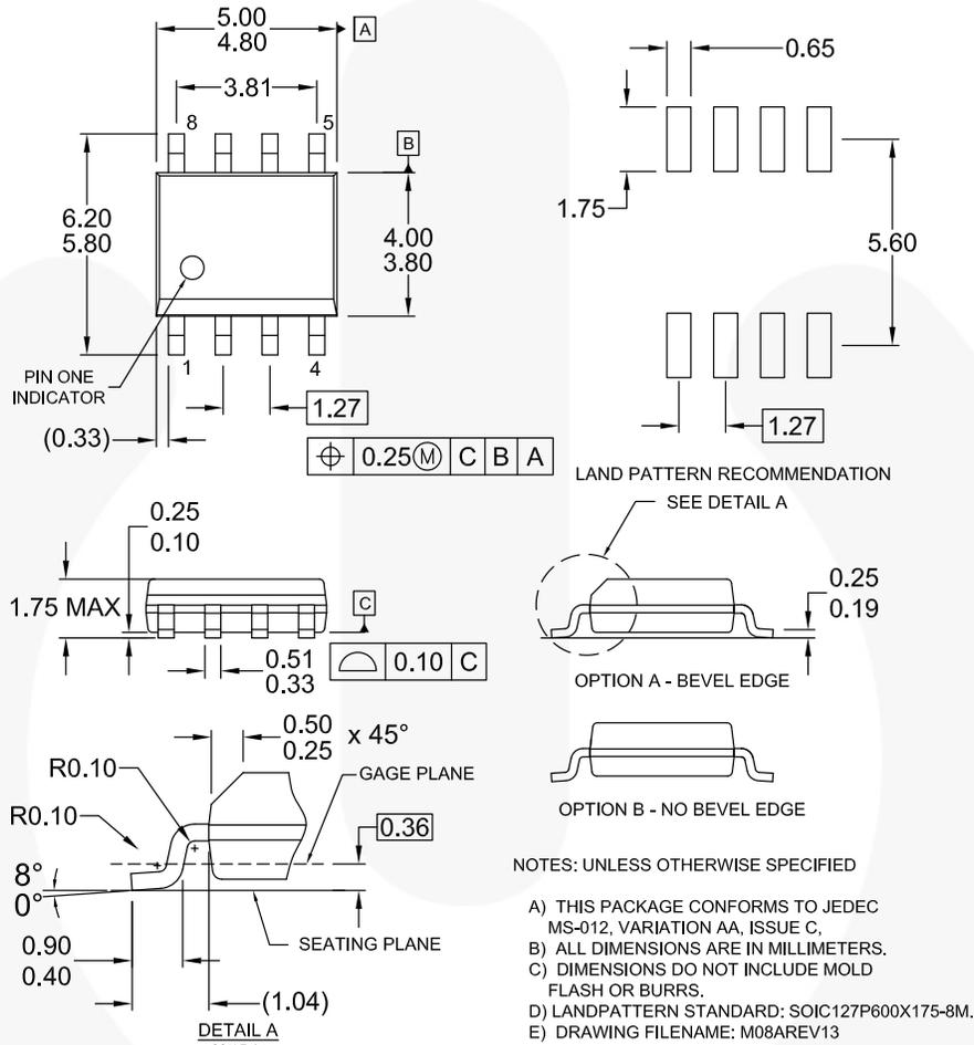
Figure 6. 8-Lead, SOIC, JEDEC MS-012, 0.150" NARROW BODY
