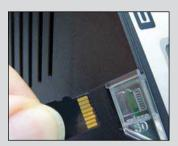
Micro smart SD card for parameterization of the i-CON pico
