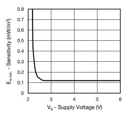
Fig. 12 - Sensitivity vs. Supply Voltage
