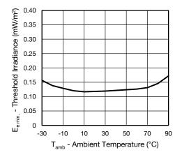
Fig. 9 - Sensitivity vs. Ambient Temperature
