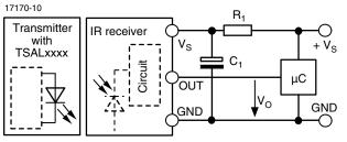
The external components R<sub>1</sub> and C<sub>1</sub> are optional to improve the robustness against electrical overstress (typical values are R<sub>1</sub> = 100  $\Omega$ , C<sub>1</sub> = 0.1  $\mu$ F).
