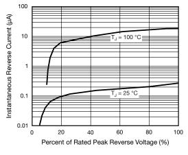
Fig. 5 - Typical Reverse Characteristics
