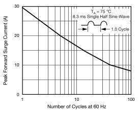
Fig. 3 - Maximum Non-repetitive Peak Forward Surge Current
