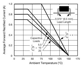
Fig. 1 - Forward Current Derating Curves
