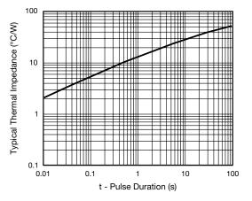
Fig. 7 - Typical Transient Thermal Impedance
