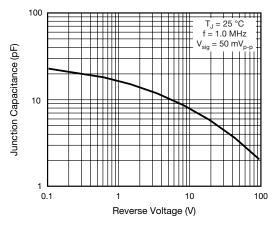
Fig. 6 - Typical Junction Capacitance
