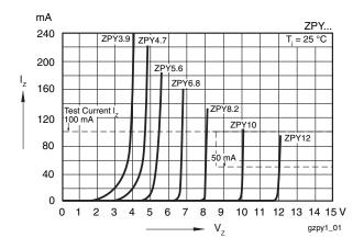
Fig. 7 - Breakdown Characteristics
