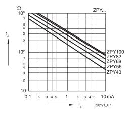
Fig. 4 - Dynamic Resistance vs. Zener Current
