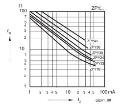
Fig. 5 - Dynamic Resistance vs. Zener Current
