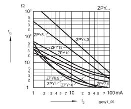
Fig. 3 - Dynamic Resistance vs. Zener Current
