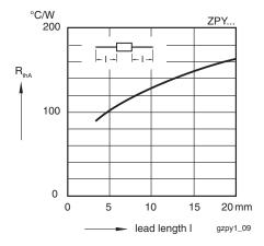
Fig. 6 - Thermal Resistance vs. Lead Length
