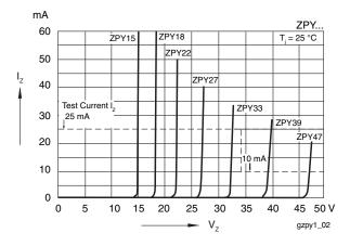
Fig. 8 - Breakdown Characteristics
