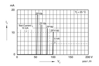
Fig. 9 - Breakdown Characteristics
