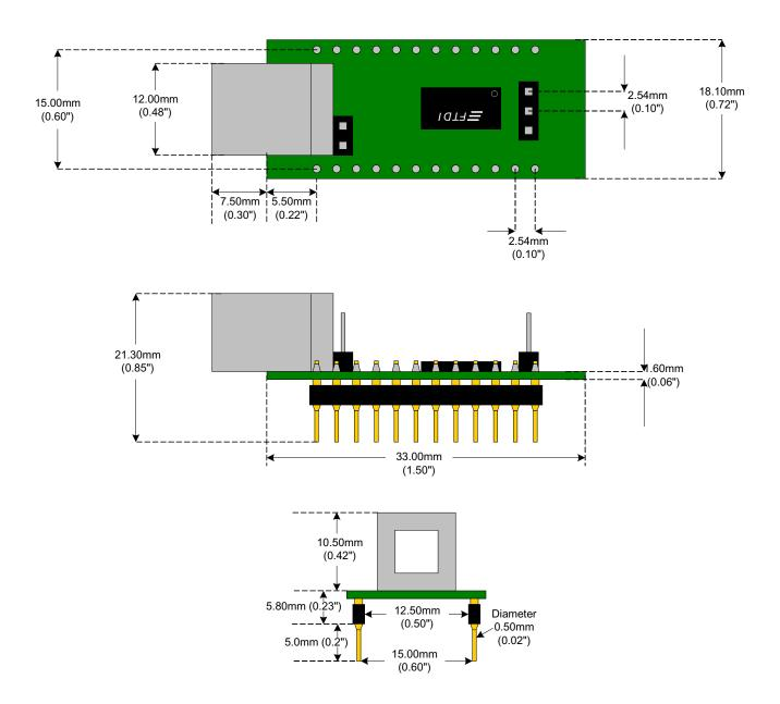
All dimensions are in millimeters, with inches in parenthesis.
