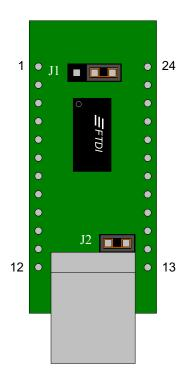
Figure 4 - Bus Powered Configuration
