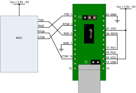
Figure 5 - Self Powered Configuration
